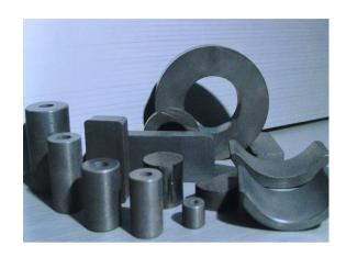
Anisotropic grades are oriented in the manufacturing direction, and must be magnetized in the direction of orientation. Isotropic grades are not oriented and can be magnetized in any direction, although some degree of greater magnetic strength will be found in the pressing dimension, usually the shortest dimension.
