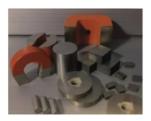
Alnico is hard and brittle. Machining or drilling can not therefore be accomplished by ordinary methods. Holes are usually cored in at the foundry, and magnets are cast close to final size and then finish machined to closer tolerances.
